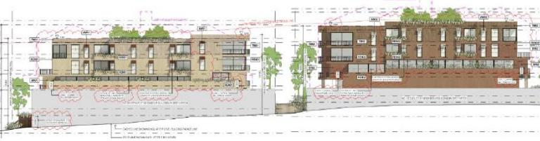
Figure 4 - Frontage to Dudley Street (to left) and Arthur Street (to east) - note ground level is different at north and south-as evident in figures 2 and 3.
